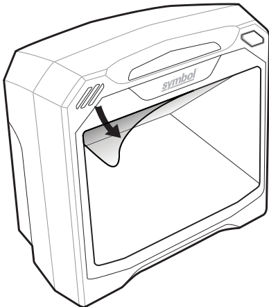
Figure 1-1 Peeling Off Protective Covering
