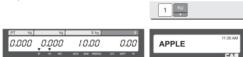
② Place an item on the platter and press the V1 key. This transaction is save to memory.
