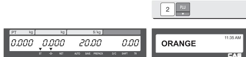
④ Place an item on the platter and press the V1 key. This transaction is saved to memory.
