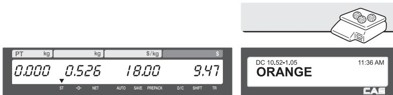
④ Place items on the platter. In this case, the weight of items(1.076kg) is greater than 2nd target(1.000kg) therefore you can have 20% discount. (Total price is 17.22)
