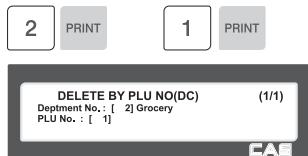
Note: There is no confirmation request when deleting a Discount of a PLU No. Pressing the PRINT key will cause the Discount of the PLU No. entered to be deleted.
