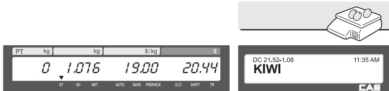
⑤ Press the PRINT key. Markdown(STRIKE THROUGH) is printed on label as figure.
