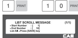
After Message No.'s are listed on the screen, pressing the TEST key will print the Message No.'s.
