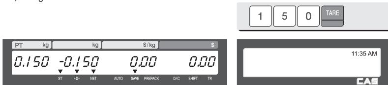
② Enter the weight of container using numeric keys.
