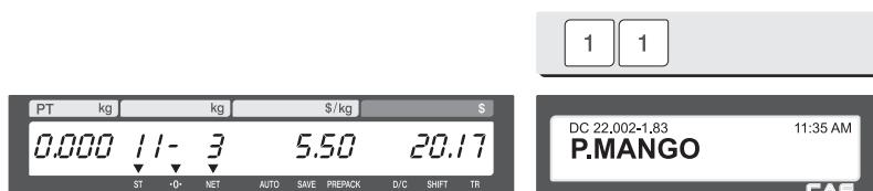
④ Press the PRINT key. Markdown (STRIKE THROUGH)s printed on label as figure.
