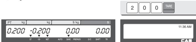
③ Press "TARE key after removing item and container from the platter.
