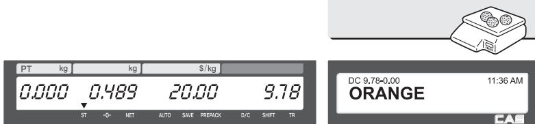
③ Place items on the platter. In this case, the weight of items(0.526 kg) is greater than 1st target(0.500 kg) therefore you can have 10% discount. (Total price is 9.47)
