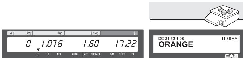
⑤ Press the PRINT key. Markdown(STRIKE THROUGH) is printed on label as figure.
