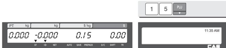
**Note:** Even though you do not press PLU key after entering a PLU number, PLU will be displayed depending on the setting time. It takes time to call up a PLU depending on the setting of parameter, 586 "Indirect PLU Call Time".
